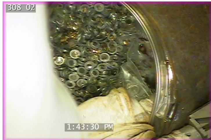
Mexican Americium source foils and sources in CPP 659 Hot Cell.
